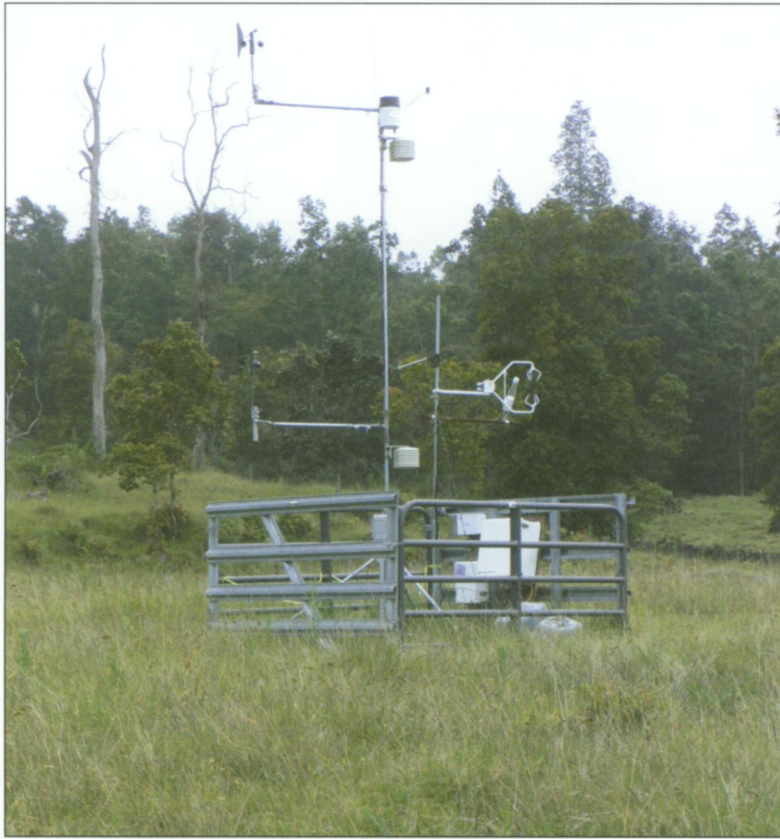
Figure 3. A micrometeorological station for quantifying the roles of pasture and nearby forest in recharging groundwater supplies for local water users. Palani Ranch, Kona, Hawai'i.
